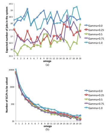
Fig. 3. Effect of  $\omega$ . Results for the criss-cross network of Fig. 1 under the traffic case B.H. and different values of  $\Gamma$  and  $\Omega$ . (a) Effect of  $\omega$  on the performance of RFP. (b) Effect of  $\omega$  on reducing the number of times we solve Problem (11). Note that the *y*-axis is in a logarithmic scale.
